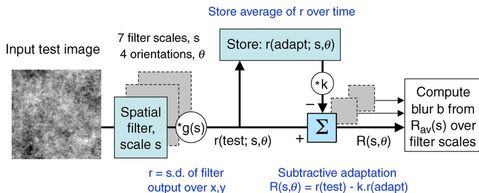
Figure 6. A sketch of the multi-scale model for blur adaptation. There were 7 filter scales, at 4 orientations. Strength of adaptation is controlled by factor  $k$ . Blur is coded from the way the adapted response  $R$  rises or falls across scales. See text for details.
